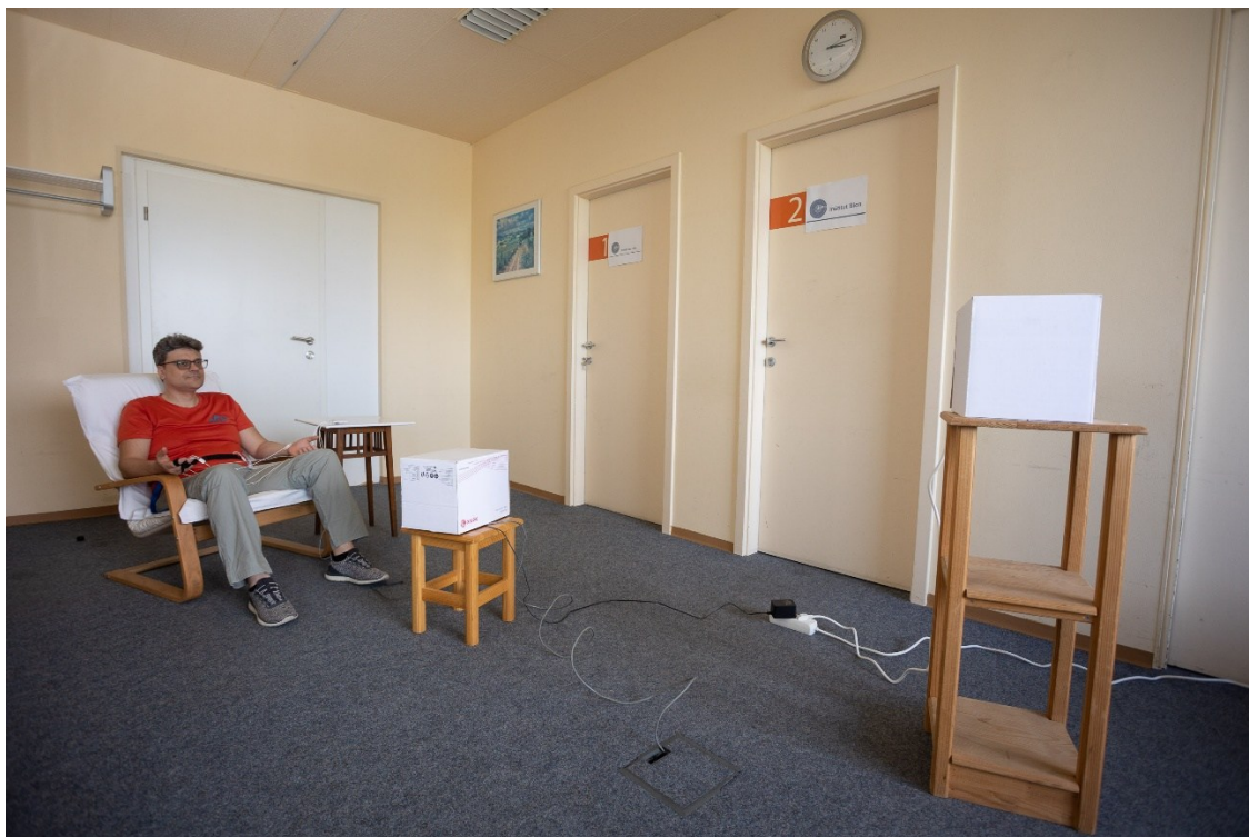
Figure 2: Demonstration of an actual testing situation. Both devices are covered by a cardboard box so that neither the assistant nor the test taker can know which situation is being performed. In addition, the test subjects do not know what is under the box.
