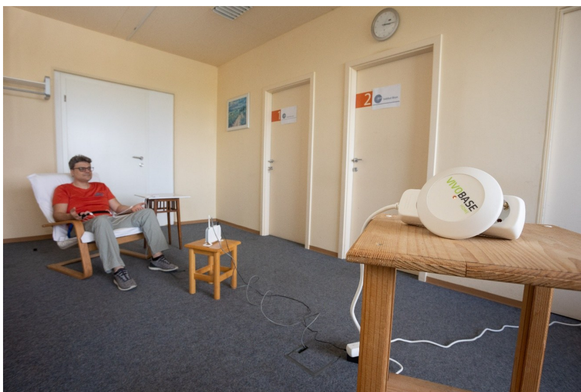
Figure 3: Demonstration of the test session with uncovered Wi-Fi router and the Vivobase Home device. As seen in Figure, both are connected to electricity. The Wi-Fi router is connected to the internet. The activation of both is monitored by
